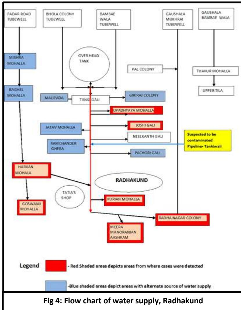
The pipeline from Bhola colony tube well (near public toilets) and tube well No.2 (near Bamba/ canal) runs independently for about 800 meters and then join together near water overhead tank into a single broader pipeline called “*tankiwali pipeline*” which supplies most of the area of the town (about 750 houses out of 1209 houses) including the areas where most of the local and tourist cases were residing. This is the oldest pipeline in the town dating more than 35 years back.
